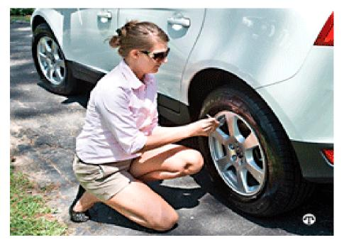
examining tires for proper inflation, dam- tread, also look for signs of uneven wear or damage such as cuts, cracks, splits, punctures and bulges. These conditions shorten the life of tires and, if not cor-• Treading firmly. The only piece of rected, may do further damage to the tire, or air loss may occur.
